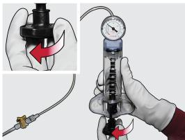
To gradually deflate, leave the locking lever in the **CENTER** position and turn the plunger counterclockwise until you have reached the desired deflation pressure.
