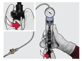
Turn the plunger clockwise until you have reached the desired pressure.
