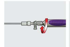
Attach the male Luer lock fitting of the connecting tube stopcock to the female luer lock fitting on the needle handle and secure tightly.
