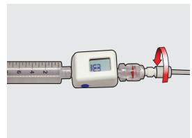
Attach the male Luer lock fitting of the transducer to the white female Luer of the connecting tube and secure tightly.
