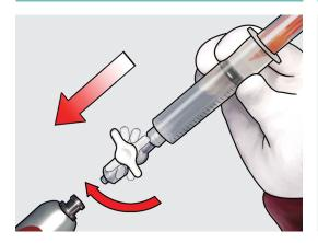
Attach the syringe to the device and open the stopcock to facilitate biopsy. Move the needle handle back and forth within the biopsy site. Upon completion of the biopsy, turn the stopcock to the closed position.
