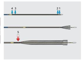
If fluoroscopically monitoring the point-of-no-return, the stent can be recaptured until the point where the external catheter radiopaque marker is aligned with the second internal catheter radiopaque marker. Note: It is not possible to recapture stent after the outer catheter radiopaque marker passes the second inner catheter radiopaque marker. Note: The stent can be recaptured a maximum of three times.
