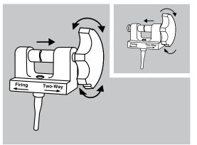
The **firing position** allows the handle to be rotated in the forward direction only. The **two-way position** allows the handle to rotate in both directions.
