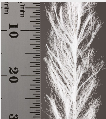
The MReye coil's extra-long fibres.
