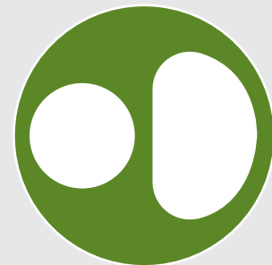
D-shaped lumen design for inflating and deflating balloon
