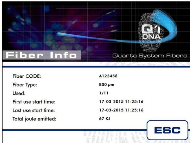
The following information of the connected fiber are stored in the internal microchip of Code Plug:
