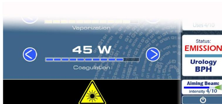
During the treatment, if the output energy fluctuates or differs more than +/- 20% from the selected initial value, then Energy Warning (Energy HIGH or LOW) is displayed accordingly. In case of Energy Warning the system does not stop, allowing in any case continuation of the treatment.
