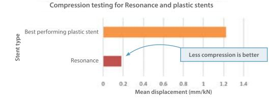
Less is better. The results of the compression testing show that the Resonance compresses less than the plastic stents tested.\*
