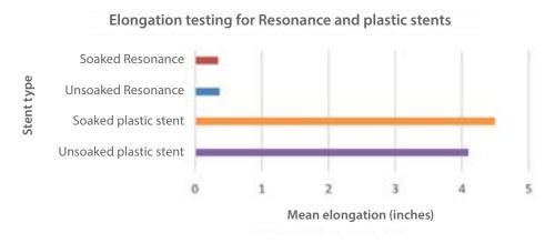
The results of the elongation testing show that the Resonance displaces less than the plastic stents tested.\*
