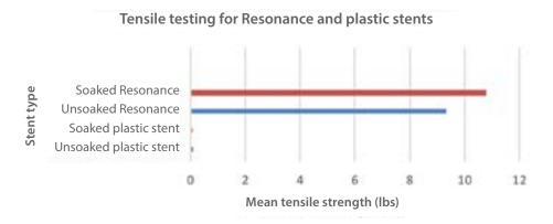
The results of the tensile strength testing show that the tensile strength for the Resonance is greater than that for the plastic stents tested.\*
