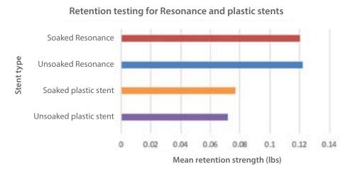
The results of the retention strength testing show that the retention strength for the Resonance is greater than that for the plastic stents tested.\*
