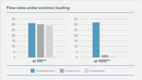
A comparative flow study shows the Resonance stent has superior flow rates to the plastic stents studied under comparable extrinsic compression testing conditions.\*\*\*
